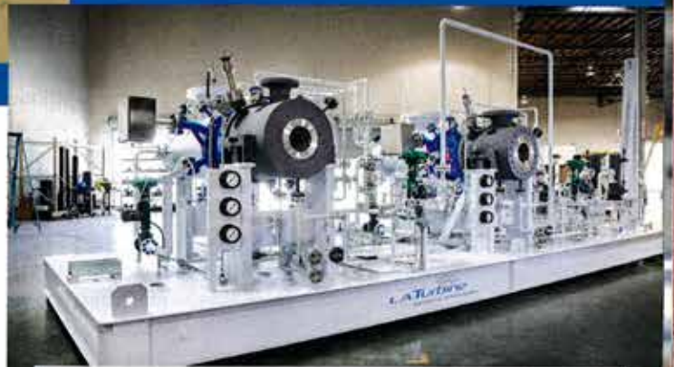
■ The LAT 560EC is L.A. Turbine's 100 th turboexpander. It is a two-stage, skid-mounted L3000 turboexpander-compressor with active magnetic bearings and a common seal gas system.
